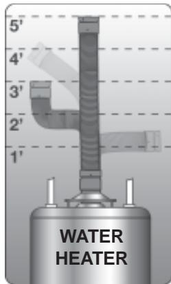
**Fig. 1 - EFC is flexible and expandable to a maximum of 60" length, permitting a variety of orientations**
