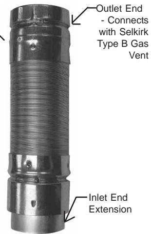
To install: Extend inlet end down over collar of appliance draft hood and secure in place with minimum 3 screws (not supplied) through the inlet end extension of the EFC and the collar of draft hood (see Figure 3). With the EFC Inlet End secured to the draft hood, extend the EFC to the required length and secure the Outlet End of the EFC to the inlet end of the Type B Gas Vent.
