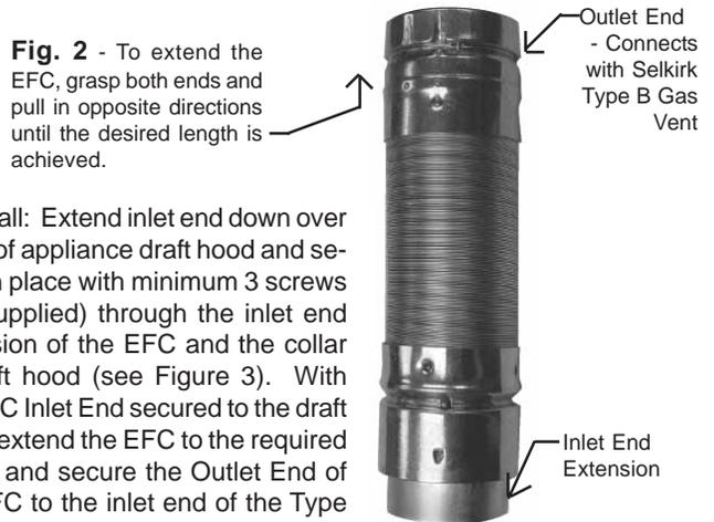
**Fig. 2 - To extend the EFC, grasp both ends and pull in opposite directions until the desired length is achieved.**
