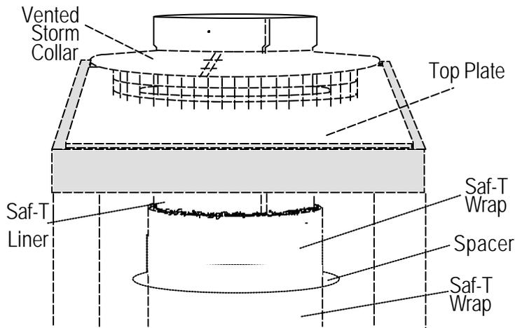
The following instructions are additions or alterations of the Saf-T Liner Installations & Maintenance Instructions and are not intended to be exclusive. To insure a safe and proper installation, follow the procedures in the enclosed Saf-T Liner Installation & Maintenance Instruction manual. Note: This system may be used to vent the flue gases of UL or other Listed appliances, with maximum continuous flue-gas outlet temperatures not to exceed 1000°F.
