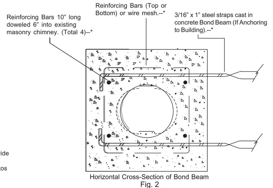
Horizontal Cross-Section of Bond Beam
