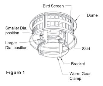
2. Ensure the Universal Gas Vent Cap is fully seated flush to the top of the Gas Vent male end. Tighten securely the worm gear clamp around the outside of the Gas Vent Pipe. See Figure 2. To remove, loosen up the worm gear clamp and lift the Universal Gas Vent Cap from the Pipe.
