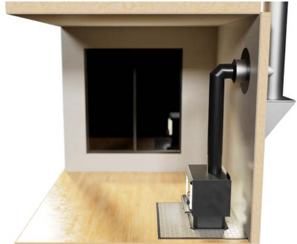
THROUGH THE WALL INSTALLATION
