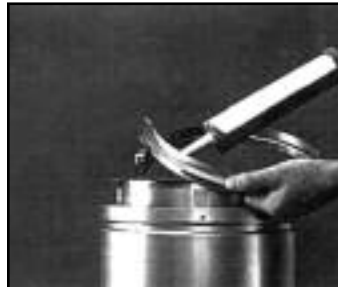
Step 1 Fill Inner Vee Band (VB) with proper sealant.
