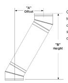
One pair of Elbows can be used to provide a sloped offset of 15° or 30°. An offset data table is supplied to determine the offset desired and the offset height.
